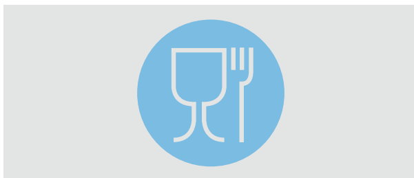
Figure 1. The ‘Glass and Fork’ symbol used to denote EU food contact compliant material.
