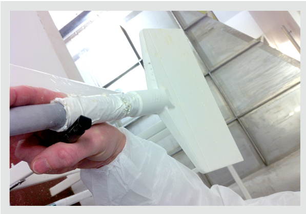
Figure 5. A scraper repaired using white plastic tape. Repairs like this increase the risk of product contamination and audit failure (courtesy of Vikan).
