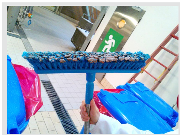
Figure 4. A badly contaminated broom in need of cleaning or replacement (courtesy of Vikan).
